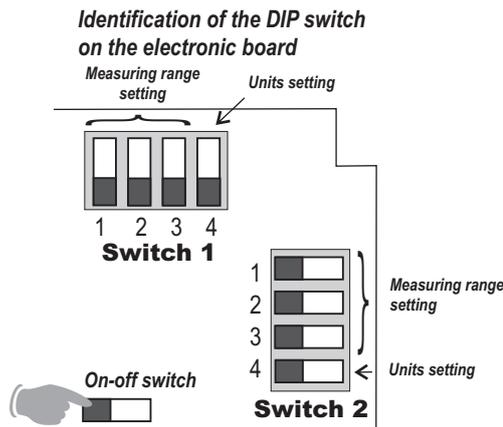
To configure the transmitter, **it must not be energized**. Then, you can make the settings required, with the DIP switches (as shown on the drawing beside). When the transmitter is configured, you can power it up.
